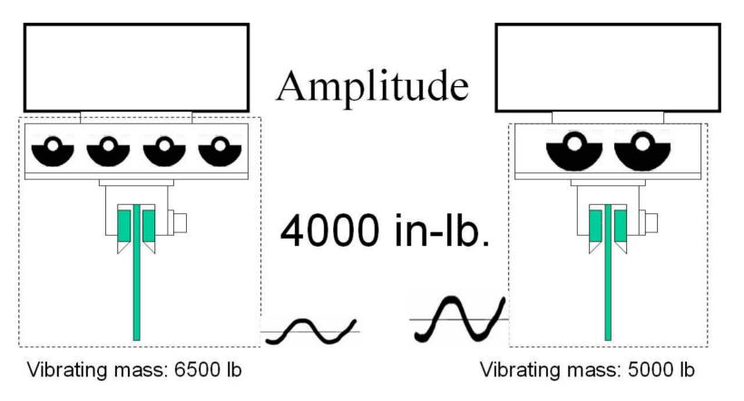
The hammer on the left has the same eccentric moment but less amplitude because the vibrating mass is heavier.
