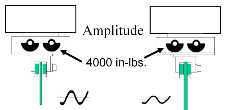
Amplitude will decrease with increase of pile weight. Big piles need bigger vibros to offset loss of amplitude.
