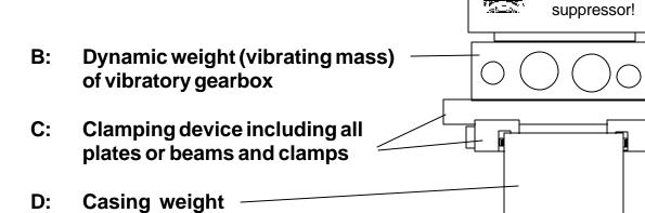
Note: Calculate casing weight using the following formula:
