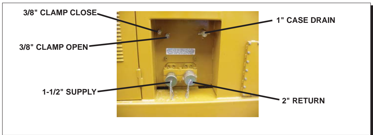
Figure 4-A. Power Unit Coupler Layout
